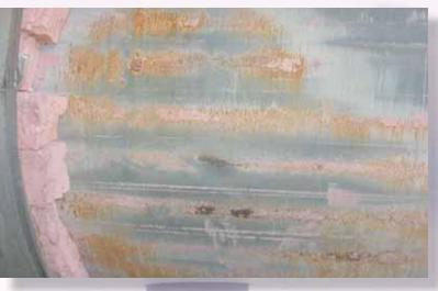
Insulation removed from a pipe originally coated with a zinc containing coating. Zinc has worked but by sacrificing, thus limiting the lifetime of the protection.
