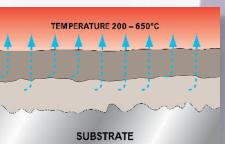
As temperature increases the moisture is drawn out of the system.
