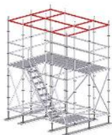
Step 10 : Connect the ledger based on dimension to the rosette of the base collar to build the third layer (second lift).
