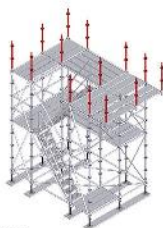
Step 16 : Put the standard to the base collar and fixed it with the locking pin.
