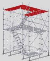
Step 13 : Put the steel plank to the ledger to built second platform based on dimension.
