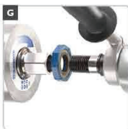
Washer quick release, to release the drill motor thread from the drill bit.
